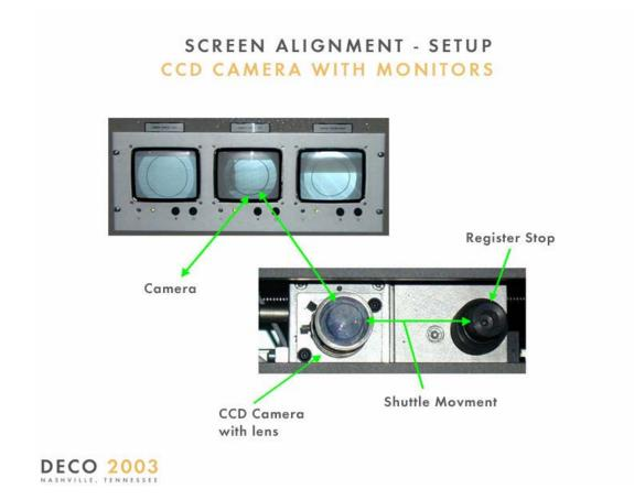
There are three "register shuttles" with CCD cameras, two along the longest side of the glass and one on the short side. The opposite sides have only the vertical positioning rollers.
